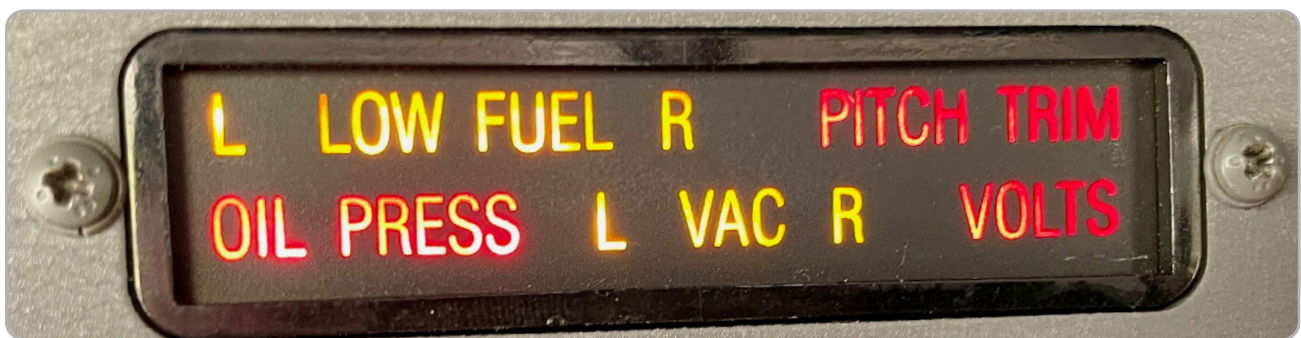
Annunciator Panel will Show L Low Fuel or Low Fuel R when 5 Gal left in the corresponding tank.
