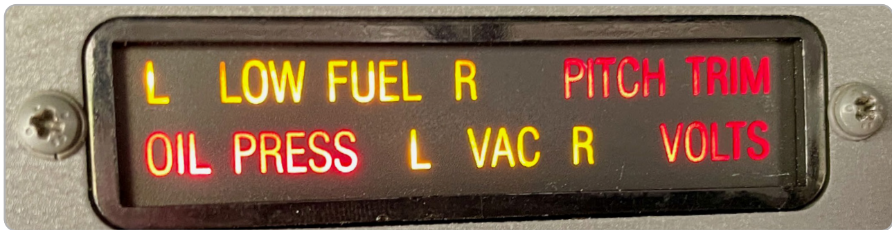
Annunciator Panel Showing Low Fuel for Both Left and Right Tanks.
